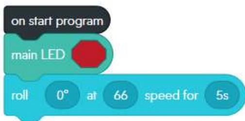
The blocks are proceeded sequentially one by one. Here the code switches the light on in red colour and then run the robot at the angle 0 by the speed 66 for 5 second.
