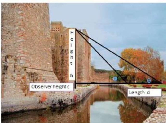
Calculating height  $h$  from two points of observation from unknown distance
